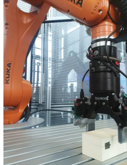
Figure 1. KUKA KR1100 sixx robot with Robotiq adaptive two-finger gripper with tactile sensors.
