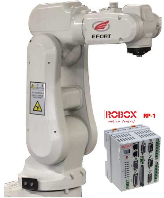
Fig. 4: Robot Efort ER3A C-60 with controller Robox RP-1
